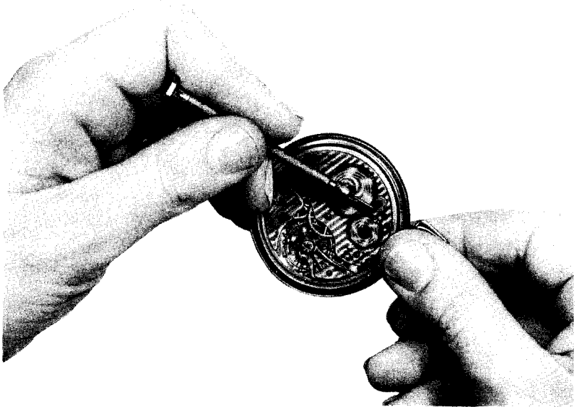
Figure 51 — Hamilton Pocket Watch — Back Removed
