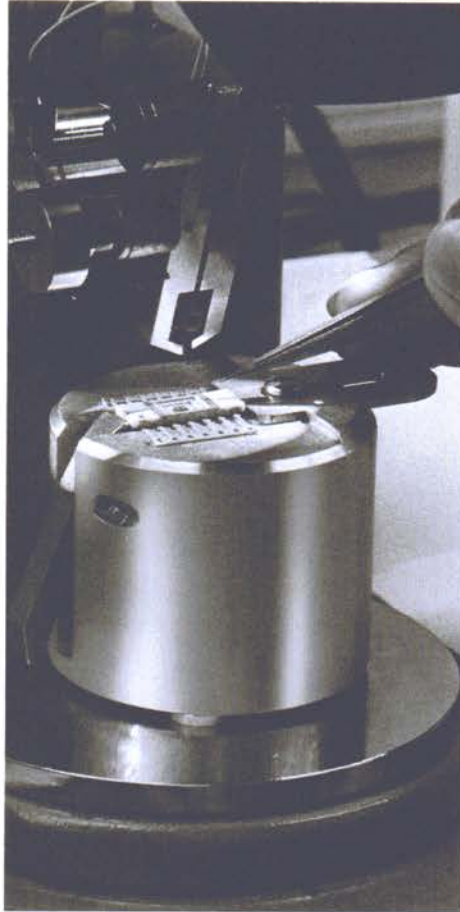
INTEGRATED CIRCUITRY—Technician prepares to attach wire leads to tiny CMOS (Complementary Metal Oxide Semiconductor) integrated circuit for solid-state timepiece.
