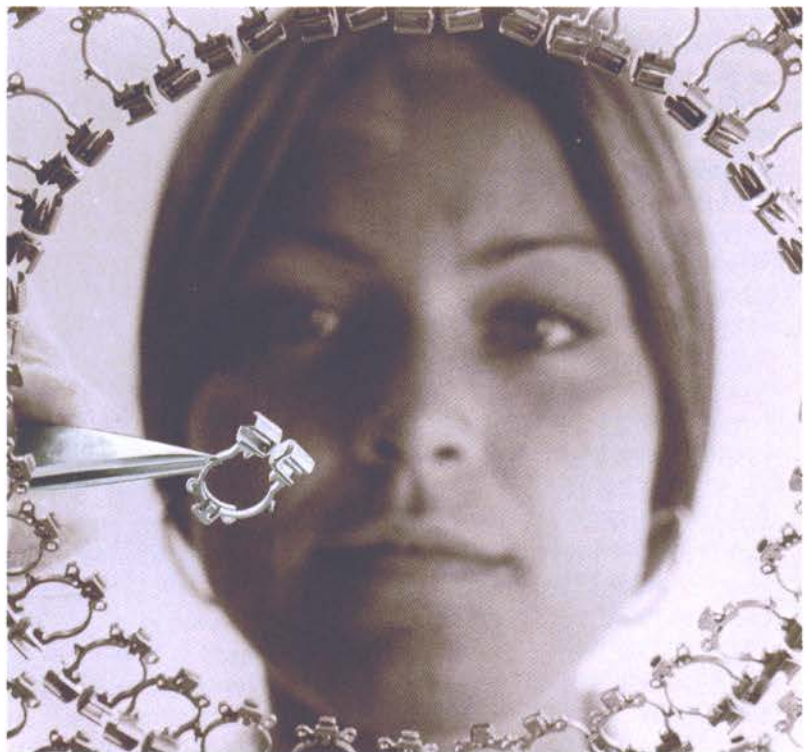
MINI FORKS —Tuning-fork inspection for Bulova Accutron woman's watches made and sold in the United States and exported to Switzerland.
