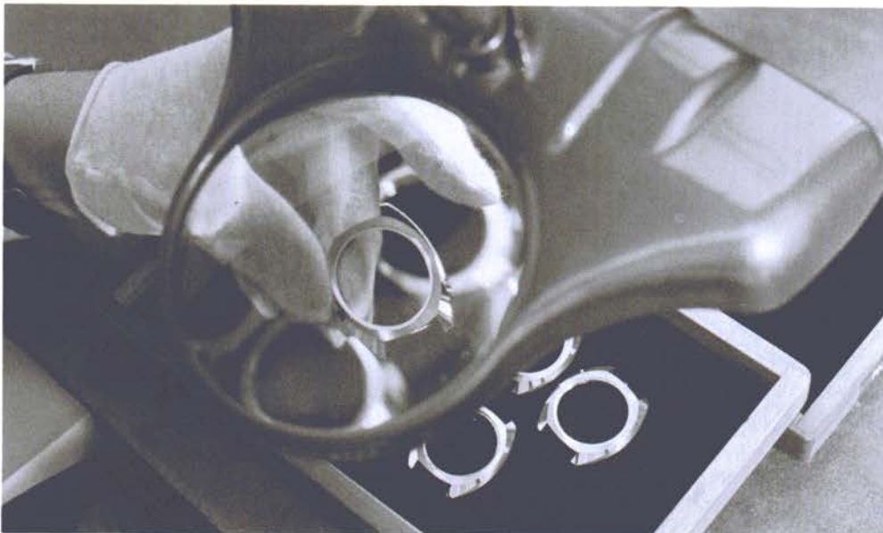
GOLD CASES—14K gold cases for Bulova Accutron men's watches are inspected by a Providence Division technician following polishing by diamond lapping.
