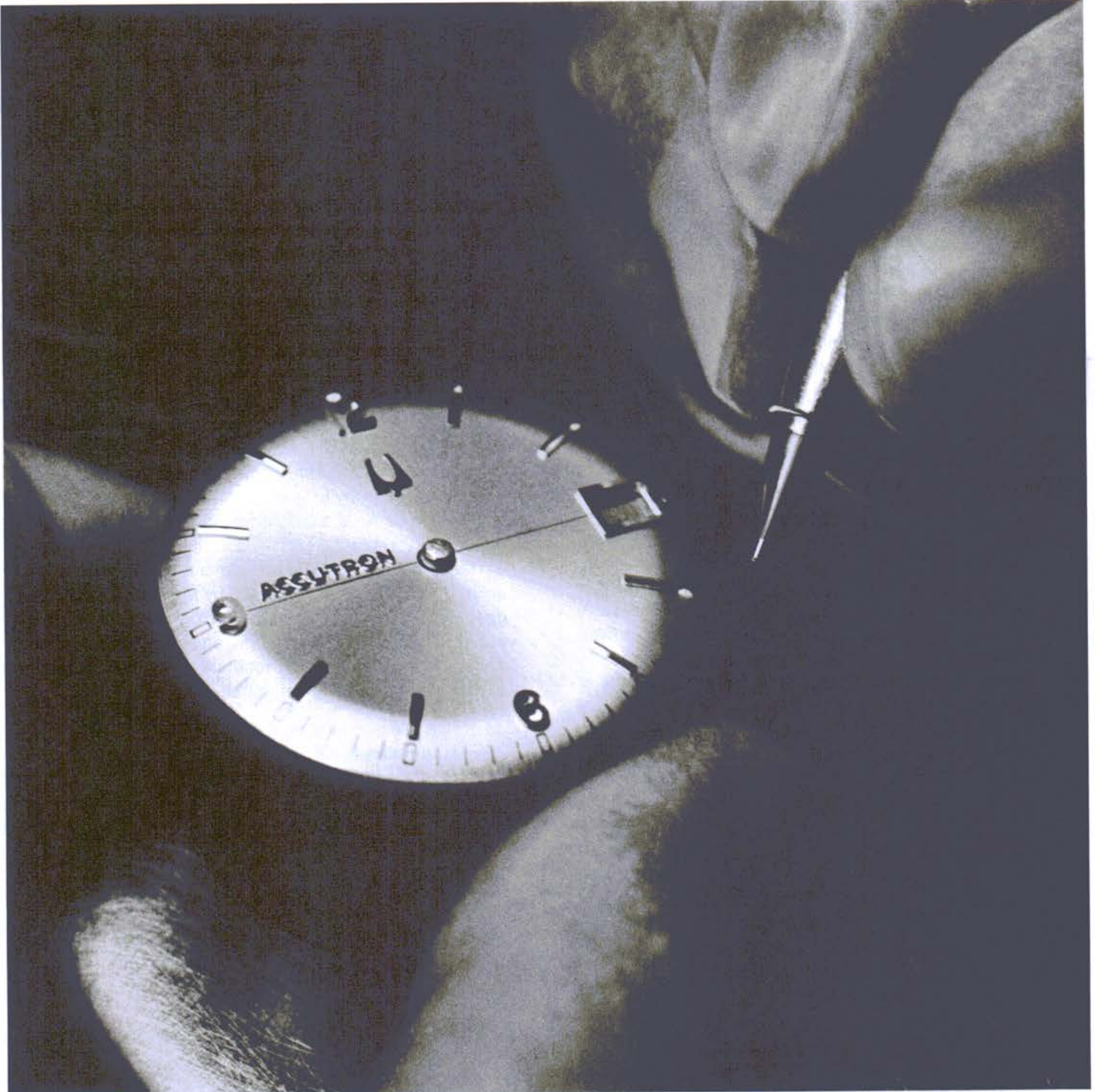
The most accurate watch in the world, the Accutron timepiece, receives hand application of luminous paint at hour markers, for utmost visibility. Shown is the dial of an Accutron date model.
