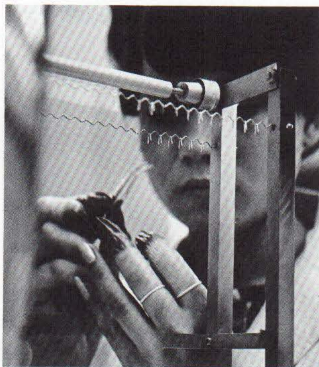
Pieces of silver of the highest purity are placed on tungsten filaments for evaporation plating of microscopically thin silver electrodes, a critical procedure in the production of quartz crystals with frequencies as high as 150 million cycles per second.
