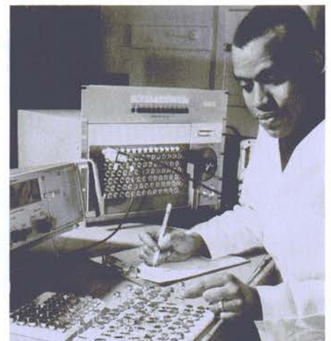
An inspector in the Electronics Division carefully measures the performance of precision crystals before shipment to customers for inclusion in advanced avionics systems.
