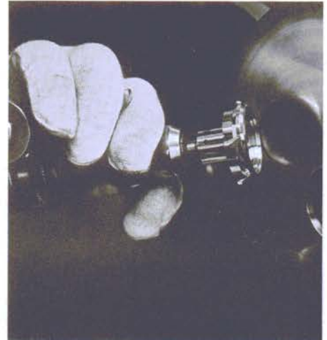
A diamond charged tin lap is used for the precision lapping of important surfaces in the production of specialized watchcases. These critical lapping operations assure sharp and precise definition of delicate facets.
