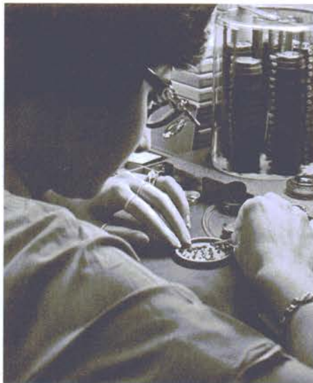
Accutron movements pass from one dust-free container to another during assembly. Shown here is a high-speed, semi-automatic indexing operation during which the movement receives a key component.
