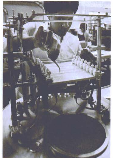
A technician at Woodside, N.Y. loads silver into an automated quartz crystal plater. Bulova's Electronics Division doubled the electrode plating capacity of the equipment to 6,000 crystals a day for use in communications, space, industrial and defense systems.
