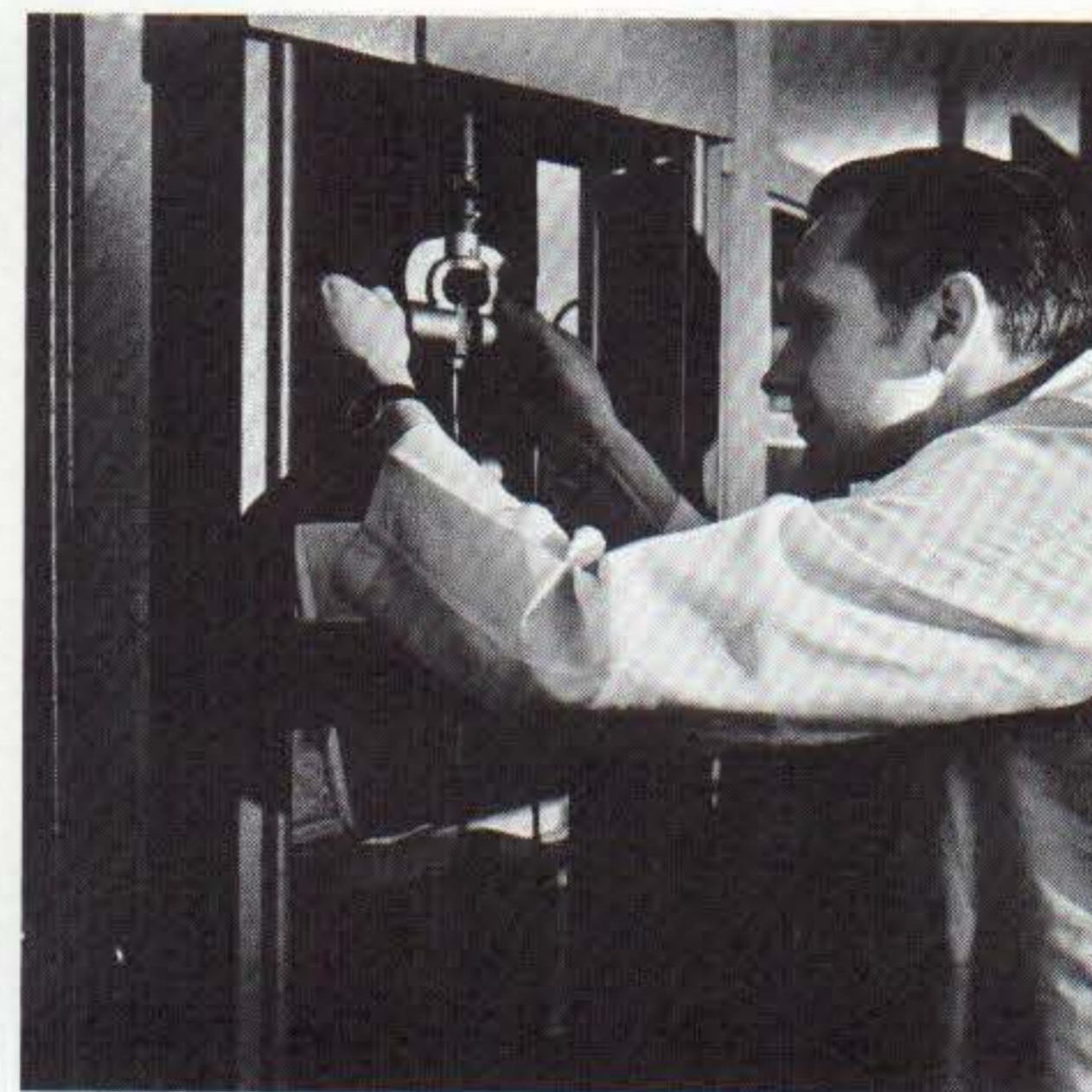
The Chemical Metallurgy Laboratory performs tests and analyses of all materials used in domestic watch manufacture. Here, electronically controlled equipment charts the tensile strength of a sampling of wire.
