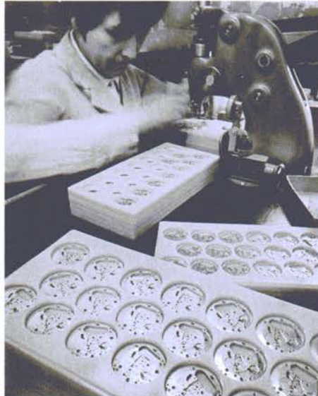
Operator of jewel setting machine performs work on pillar plates. Multiple stacking of assemblies facilitates handling.
