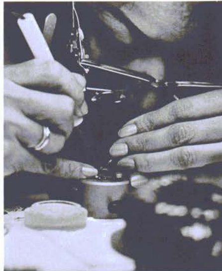
One of hundreds of procedures in the precision-assembly of the Accutron timepiece is this critical micro-soldering operation within the electronic module. The tiny electronic circuitry in the module furnishes the Accutron tuning-fork with the power to vibrate 360 times a second.
