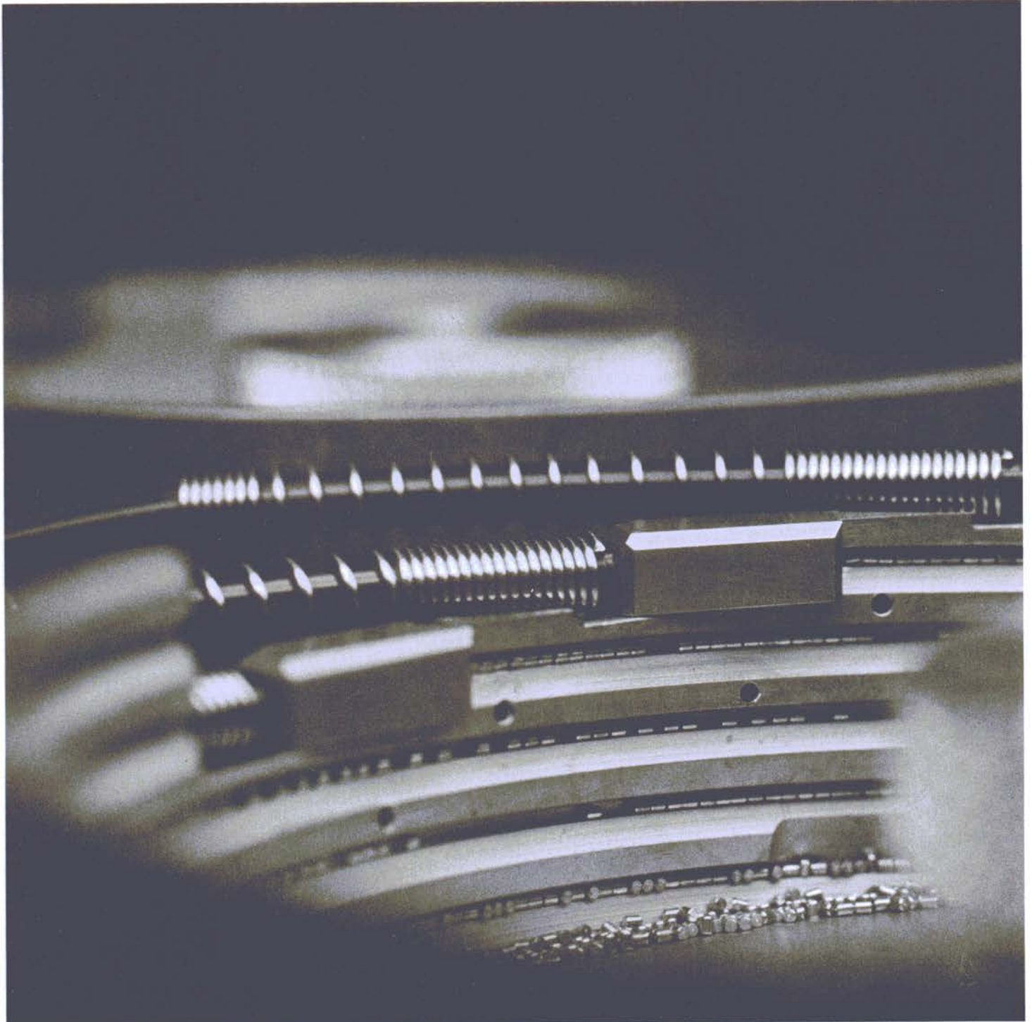
Inner view of a vibrator feeder, designed and engineered by Bulova for the automatic positioning of Accutron tuning-fork magnets and other components used in assembly.
