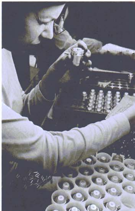
Ordnance fuzes undergo rigorous sequence of visual and mechanical inspections at Providence, R.I. Under contract to the U.S. Department of Defense, Bulova's Providence Division produces approximately 400,000 time fuzes a month.
