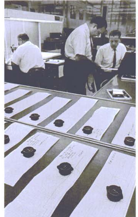
Industrial Accutron timer units are custom engineered for specific applications and are lab checked for pinpoint performance. Here, the charted results of several Accutron models are recorded to determine individual accuracy.
