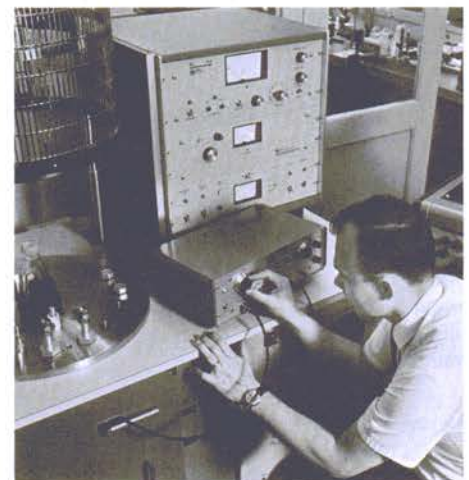
The basis of future timekeeping systems is explored in Bulova's Advanced Research Laboratory, with the aid of specialized equipment. Shown here is a high-vacuum evaporator test unit and associated multi-channel nuclear particle spectrometer.
