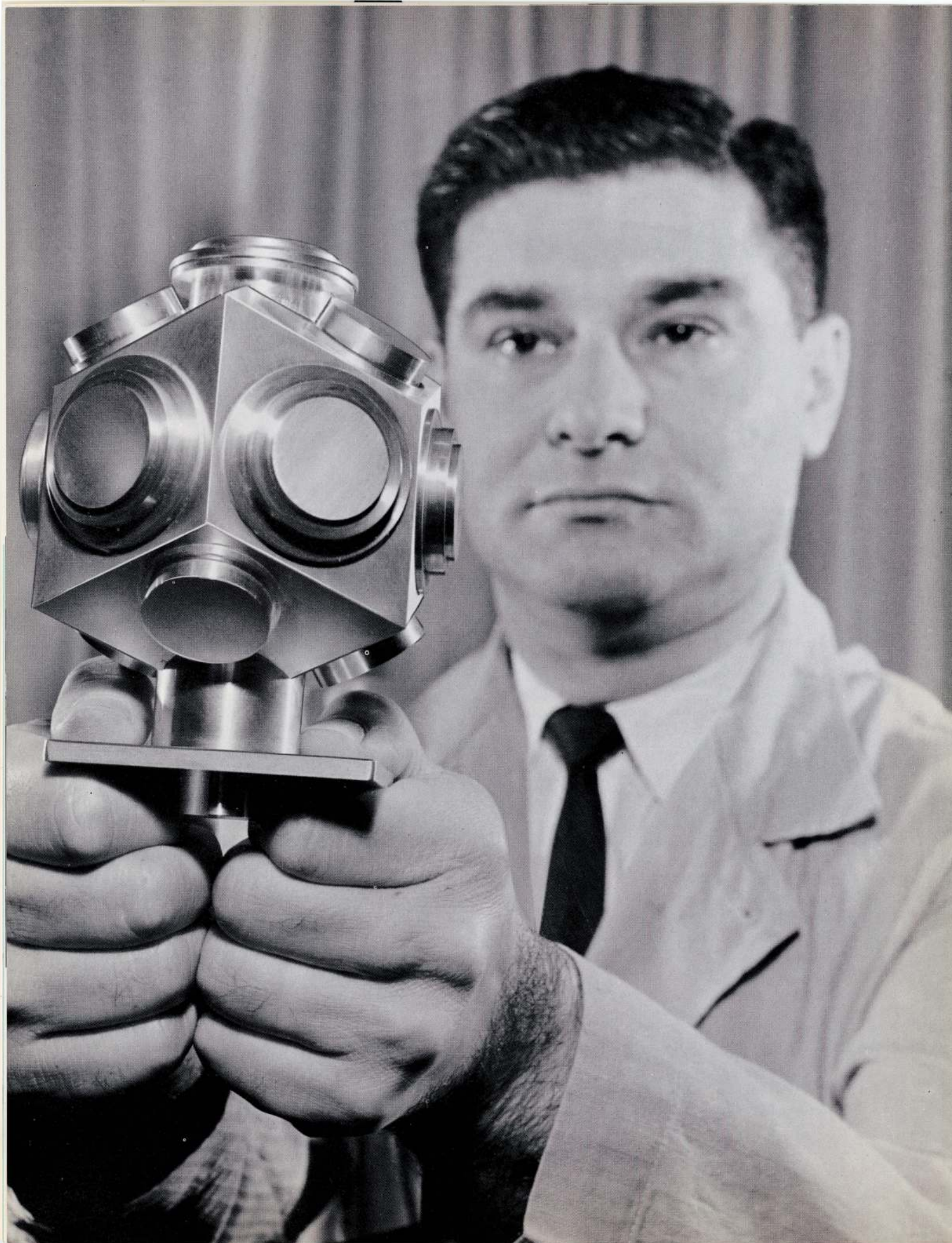
▲ Bulova engineer Marvin Marcus checks prototype model of "sun seeker" electro-optical device developed for Lockheed satellite program. Device is to keep satellite advised of its position relative to the sun, and it was specially designed so it would not be "fooled" by any other light sources in space.
