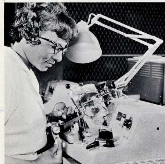
▲ Coil winding is an ancillary manufacturing process developed within the Company to assure supply and quality control of components for Bulova's electronic products.
