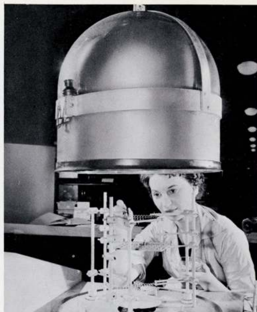
▲ Dryer-like dome is really a large bell jar used at Electronics Division during vacuum process in silver-plating step in manufacture of precision quartz crystals.
