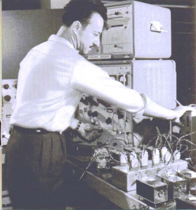
Oscillators used to establish precise frequencies for electronic components of missiles are checked on advanced test equipment in Bulova's electronics laboratories.
