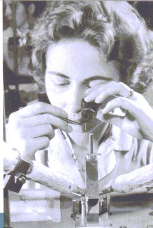
Scientific soldering of leaders is a key step in crystal production at Bulova. Hair-size leaders are soldered to the crystals by jets of nitrogen gas flame.
