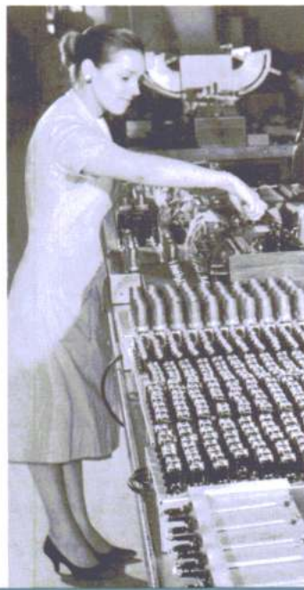
Five models of tiny, thermostatically controlled "ovens" are produced by Bulova to maintain crystals at the desired frequency for electronic applications in the missiles, defense and commercial field.
