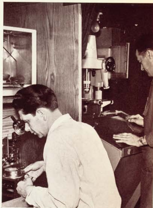
Further inspection of Escape Wheel. Machine at right projects and magnifies part 100 times on a screen, so it can be checked perfectly against a standard pattern.
