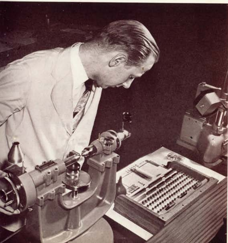
Feeding the milling machine that mills the gear teeth on pinions. Each tiny tooth must be highly polished to a smooth mirror finish to eliminate all possible friction.
