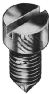
Finger Marks on Screw Head
